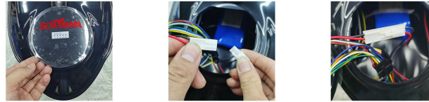
(1)Open the battery case in front. (2)Connect battery with PCB board power plug (3)Ensure two plugs connect well.
